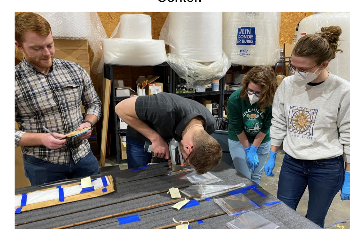
The team uses XRF to test treated ethnographic artifacts to detect the use of heavy metals by collectors.
