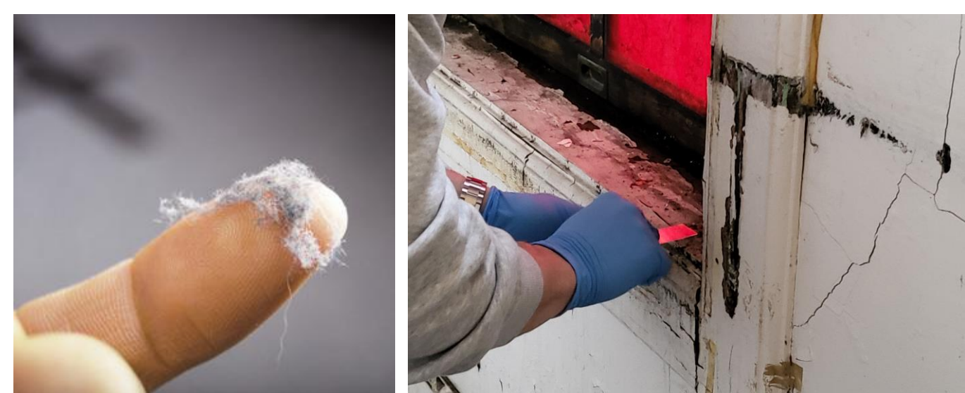
Photo credit: Livescience. Sampled a window for the presence of mold using a Bio-Tape slide
