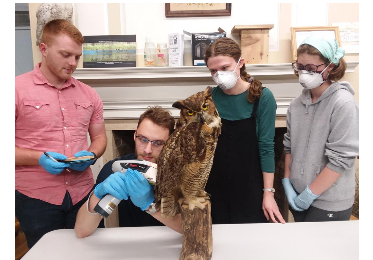
(Left to Right) K. Burnell, J. Klicker-Weichmann, E. Daugherty, and M. Griem measure the levels of arsenic present in a taxidermy mount using a portable XRF device at the Eagle Creek Ornithology Center.
